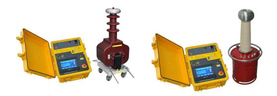
5/50 Dry testing transformer weight is about 47kg. 5/50 Gas testing transformer weight is about 40kg.
